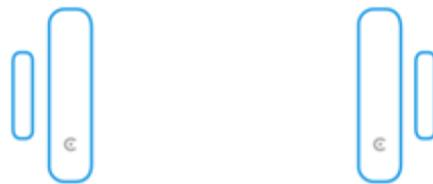
Here are a few examples of how the sensor and magnetic contact could be mounted:
